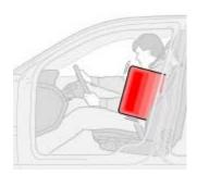
The SIPS airbag system is designed to help increase occupant protection in the event of certain side impact collisions. The SIPS airbags are designed to deploy only during certain side-impact collisions, depending on the crash severity, angle, speed and point of impact. The airbags are not designed to deploy in all side impact situations.
