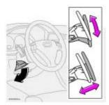
Both the height and the reach of the steering wheel can be adjusted to a comfortable position for the driver. Pull down the lever on the left of the steering column. Adjust the steering wheel to a suitable position and press the lever back into place to lock the steering wheel in the new position. Check that the steering wheel is locked in the new position.
